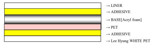
When attaching GLASS, please attach it with the WHITE PET release side.
